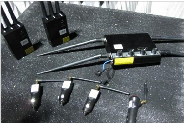
Figure 12: Jammers used in laboratory testing.
